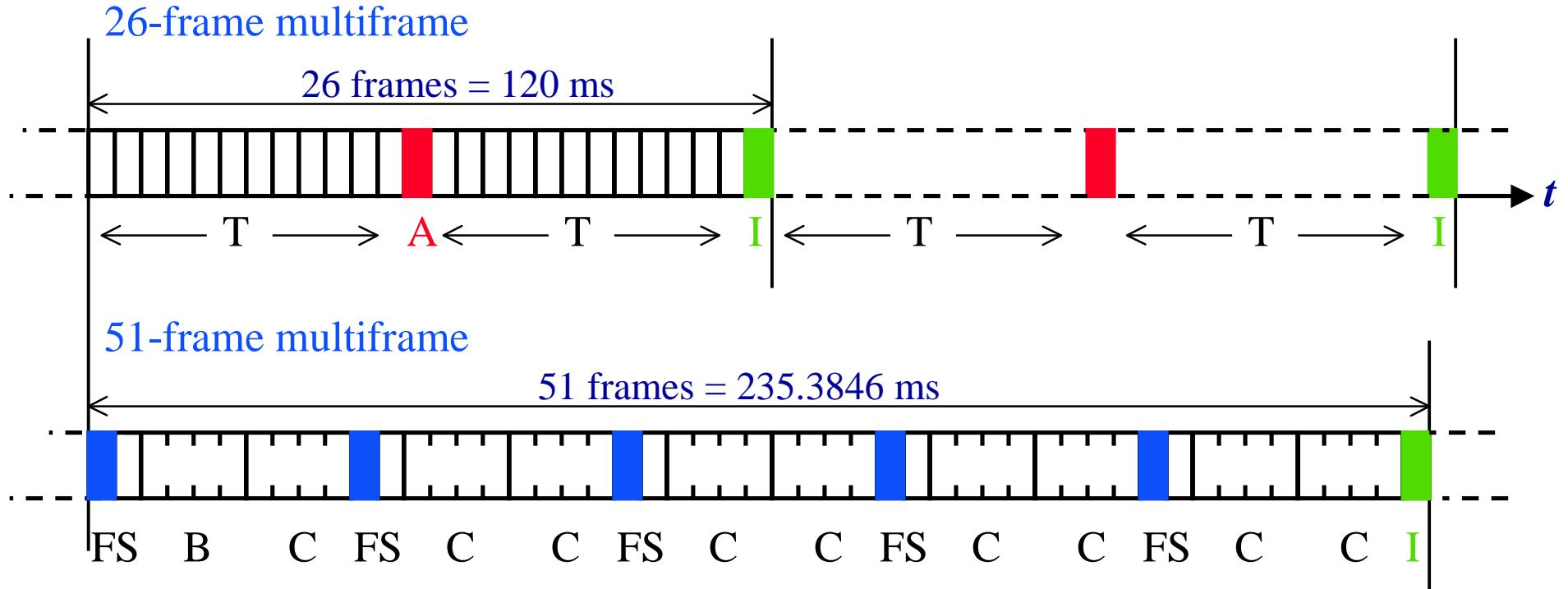
SUPERFRAME:  $51 \times 26\text{-frame multiframes} = 26 \times 51\text{-frame multiframes} = 6.12\text{s}$
