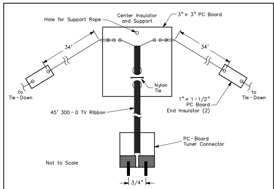
Figure 1—General construction of the 80-meter Squirt antenna.
