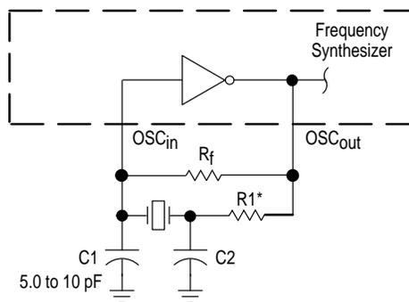
**Figure 19. Parasitic Capacitances of the Amplifier and C<sub>stray</sub>**
