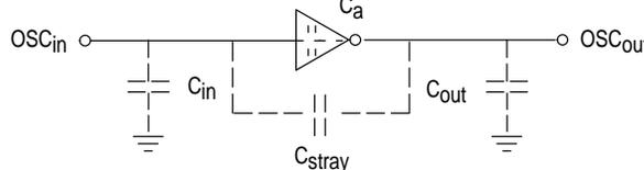
**Figure 20. Equivalent Crystal Networks**
