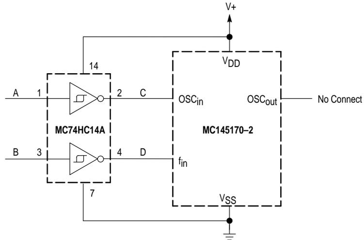
NOTE: The signals at Points A and B may be low-frequency sinusoidal or square waves with slow edge rates or noisy signal edges. At Points C and D, the signals are cleaned up, have sharp edge rates, and rail-to-rail signal swings. With signals as described at Points C and D, the MC145170-2 is guaranteed to operate down to a frequency as low as dc. Refer to the MC74HC14A data sheet for input switching levels and hysteresis voltage range.
