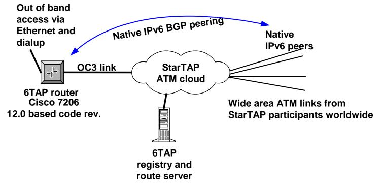
R&E network already using v4 over ATM to reach StarTAP simply sets up a v6 ATM PVC path to the 6TAP router
