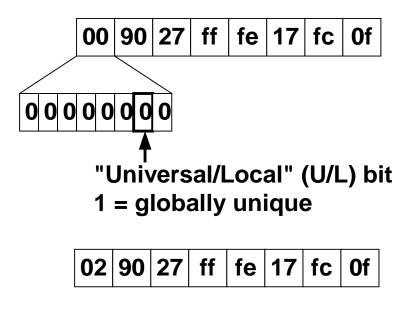
So lower 64 bits in address are 02:90:27:ff:fe:17:fc:0f
