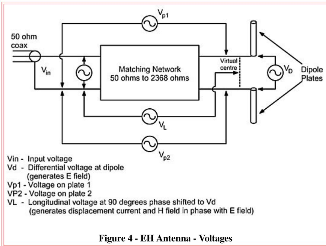
**Figure 4 - EH Antenna - Voltages**
