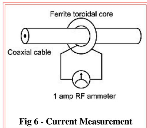
**Fig 6 - Current Measurement**
