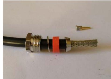
Over the cut end of RG58 coax slide the clamp nut, washer, and seal. Strip the sheath off over-long (approx. 15mm) and slide on the tapered collet.
