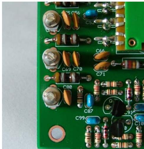
R2 PA bias current – disconnect the antenna and connect a dummy load suitable for 5 Watts. Connect an ammeter in series with the radio and power supply capable of reading 3 amps. Whilst making this adjustment do not speak or make other noises into the microphone; press
