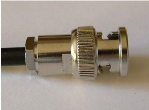
Fit body and tighten clamp nut, finally check that there is no short circuit between inner and outer contacts and that inner contact is in correct position.
