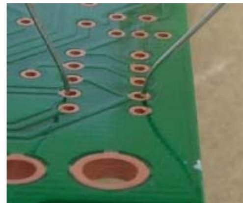
become confused (especially zener diodes and trimmer capacitors). Everyone has their preferred method of retaining components prior to soldering; I pull the leads through with long nose pliers and put a bend in the component lead to stop it falling out of
