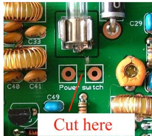
The PCB incorporates a facility for fitting a power switch, the RF gain control may be replaced by a switched 4k7 linear potentiometer and the power switch wired to the marked pads. For the switch to function the track needs to be cut with a sharp knife where indicated.
