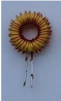
L1 and L4 – Cut off approximately 40cm of 27 SWG wire and pass half of it through the center of a T37-6 core, this counts as the first turn. Now wind a further 14 turns through the core using one end of the wire, turn the core over and wind the other end through the core 15 times making a total of 30 turns. Whilst winding pull the wire tight so the turns lay touching each other. Crop the wires to 10 – 20mm in length and tin the ends with solder.
