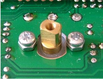
Fit the tuning capacitor using M2.5 x 6mm screws. NOTE: screws must have nuts fitted underneath their heads before fitting so as screw thread doesn't foul the capacitor vanes.
