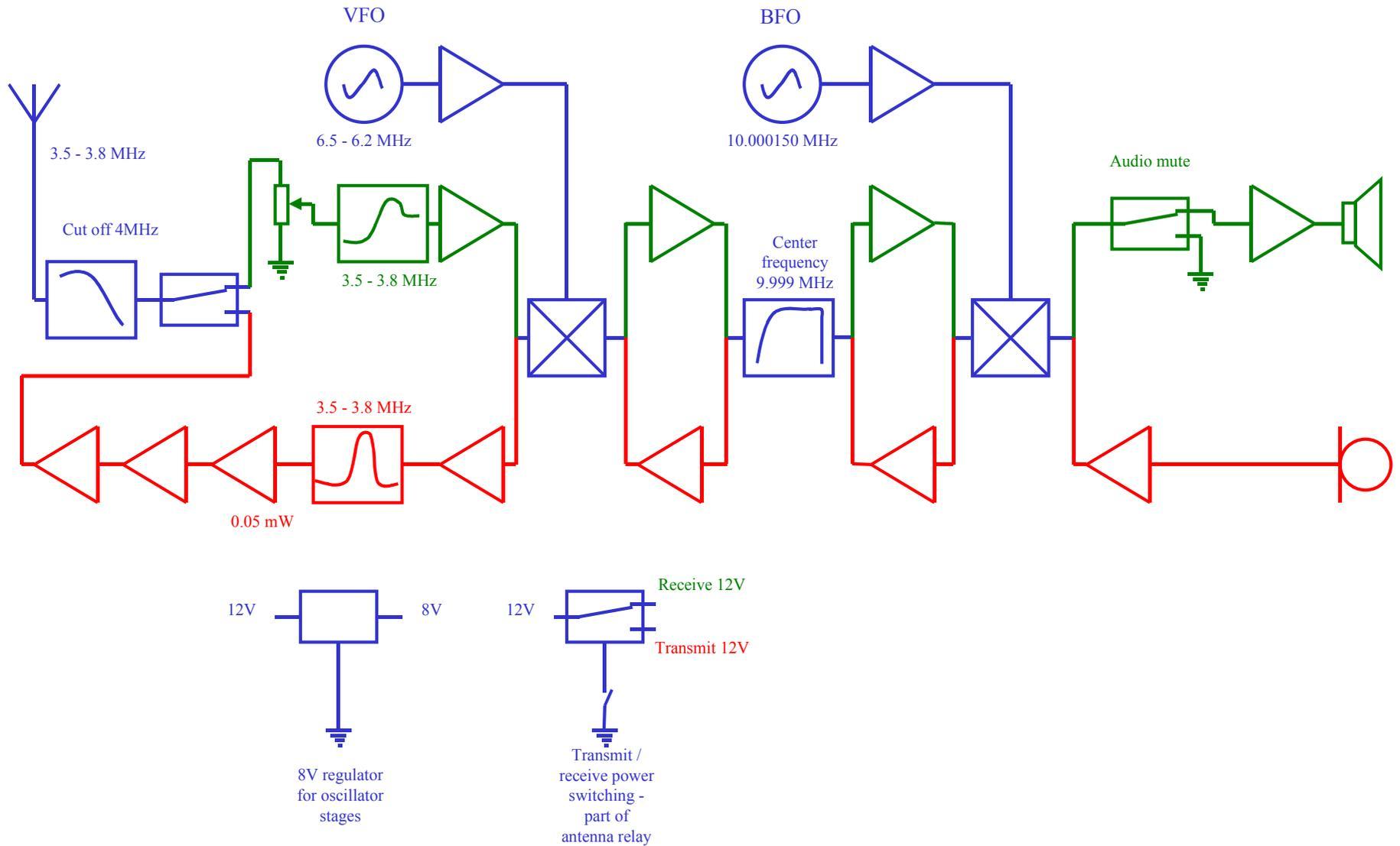
The radio uses a single IF super-heterodyne architecture with several so called bi-directional stages. These allow the sharing of all the main functional blocks between transmit and receive – mixers, IF filter VFO and BFO.
