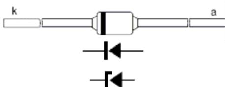
Values are marked on the bodies although for the small glass diodes (zener diodes and 1N4148 types) they will be hard to read without a magnifying glass.
