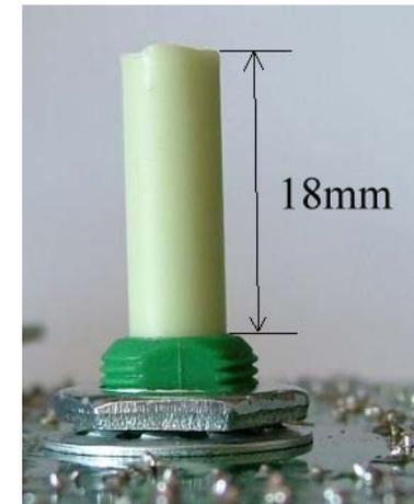
Before fitting VR1 and VR2 cut the shafts to required length, if using the suggested case the shafts need to be cut so that 18mm is left protruding above the mounting thread.
