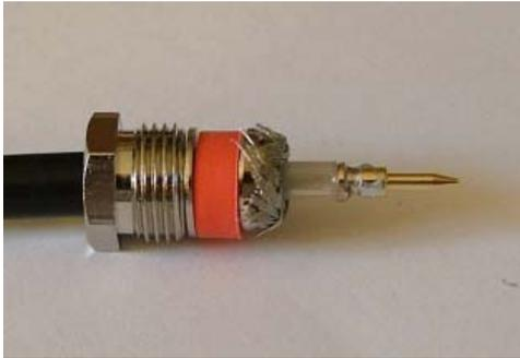
Fit the inner contact and solder through small hole.
