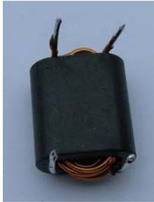
T2 is wound using the same method as for T1 and T3 but the windings have three turns of 22 SWG wire on the larger BN43-0202 core.
