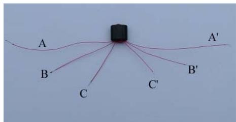
Locate the second wire, trim these two ends to about 30mm in length, and now confirm the last two ends belong to the third wire and crop to about 15mm in length. These wires are then passed through the PCB longest first and shortest last, anchor the transformer into the PCB by bending 4 wires over
