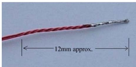
Thread the soldered end through one of the holes of a BN43 – 2402 core (the smallest core, see photo) leaving about 10cm remaining then thread the wire back through the other hole – this is one complete turn. Loop the soldered end through a further 4 times to make a total of 5 turns. Trim the wires back to about 50mm in length, splay apart and tin the ends with solder.
