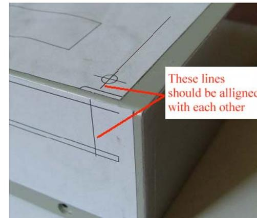
To cut the display window without special tools I would recommend drilling many holes close to each other just on the inside of the window then using a pair of side cutters join them up. The window can then be squared up using a file.
