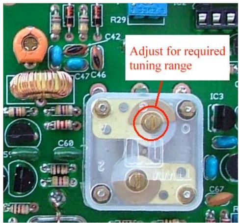
Polyvaricon (VFO) to maximum frequency and check that it is possible to tune above the top of the band. If desired the total tuning range can be adjusted with a trimmer capacitor on the back of the Polyvaricon. Moving the capacitor into mesh will reduce the range and moving
