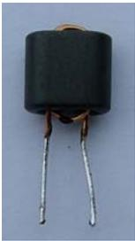
L3 – wind 2 turns of 27 SWG wire through the holes of a BN43-2402 core and tin the leads.
