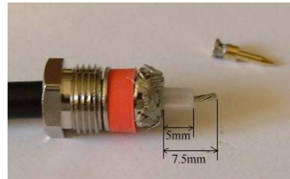
Pull braid back over tapered collet and trim; trim the inner conductor length to 7.5mm and then strip the dielectric to 5mm in length.
