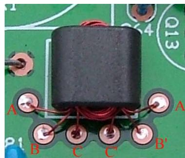
into position with a little non-acidic silicon adhesive, note that bathroom sealer is not suitable as it exudes acetic acid whilst curing. The correct adhesive doesn't have any smell.
