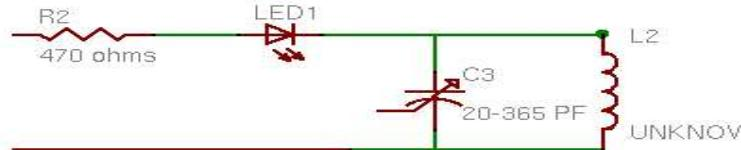
Connect your RF source to the left side of this circuit and tune the variable capacitor for a dip in the LED brightness (look close, some LEDs do not show much light output).
