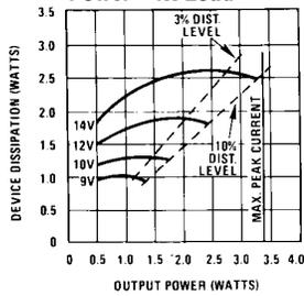
**Device Dissipation vs Output Power— $8\Omega$  Load**
