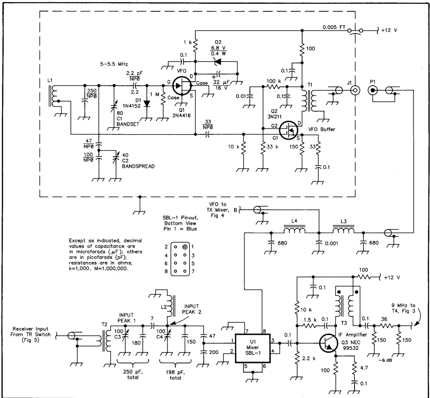
Fig 2—Schematic of the transceiver front end and VFO. Resistors are 1/4 W, carbon film; unless otherwise indicated, capacitors are monolithic or disc ceramic. The VFO circuitry is built into a die-cast aluminum box.
