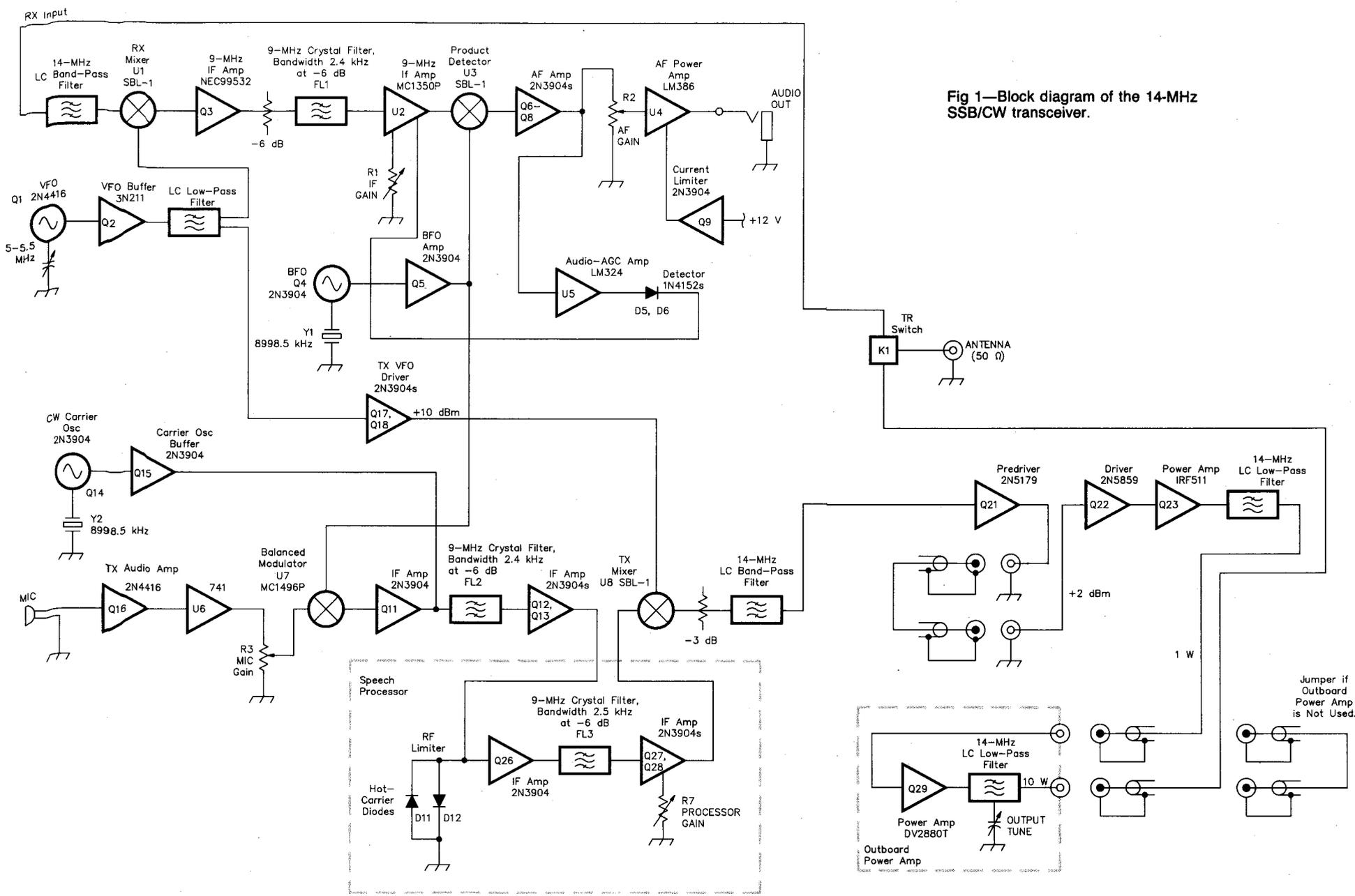
Fig 1—Block diagram of the 14-MHz SSB/CW transceiver.
